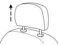
2. Use a push tool, such as a key, to press the small button located on the side of the guide sleeve and, at the same time, press the lock/release button, then pull the head restraint upward.
